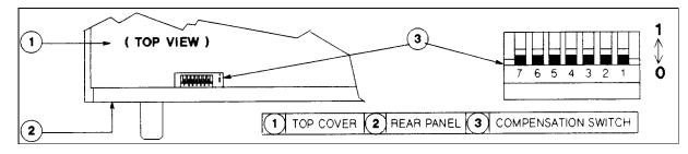
Figure E-2. CC Loop Compensation Switch
